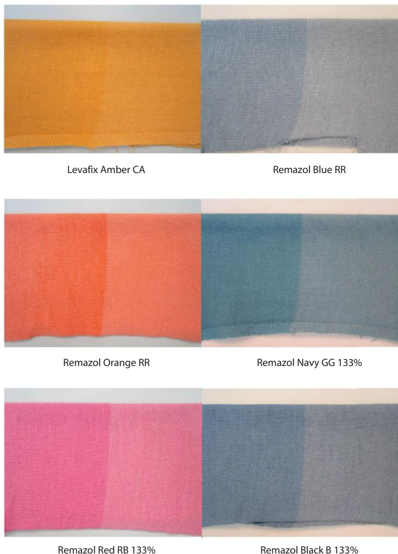
Figure 5.12 Cotton knitweaves made from yarns submitted to free UV treatment (reprinted from Migliavacca [11]).
